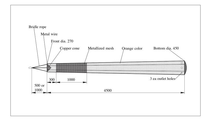
The sleeve target has a slight conical shape. It is manufactured of PVC coated fabric. It consists of a circular half spheric end, and two longitudinal orange colored gores.
