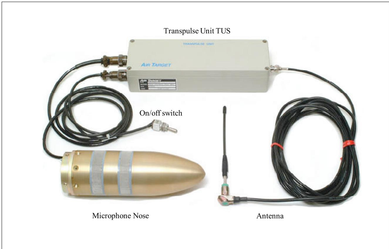
The universal 12-sector Miss Distance Indicator MDI AS-133/12U is intended to be installed in both hard targets and UAVs (Unmanned Aerial Vehicles).
