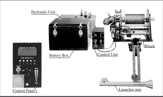
Winch, hydraulic unit, battery box, launcher arm, control panel and control unit.
