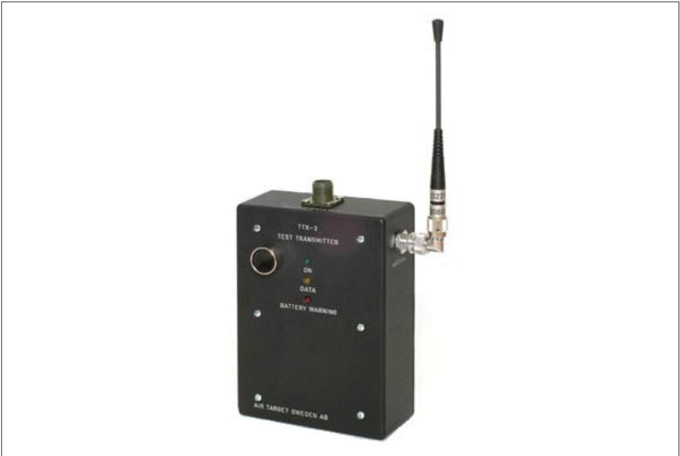
The test transmitter TTX-3 is a battery operated transmitter unit to check the function of the Marque, Mini Marque and VDU-12 scoring stations. It is designed to produce the same signals as those from a miss distance indicator of the AS-100 family with 2-level FSK telemetry and CRC checksum.
