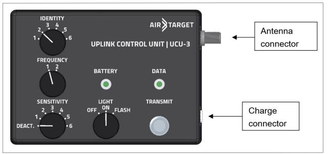
The Uplink Command Unit UCU-3 is is a handy battery powered unit for transmitting commands to the Miss Distance Indicator (MDI) equipped with an uplink receiver.
