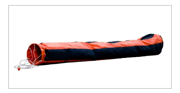
The sleeve target has a slight conical shape. It is manufactured of a thin, light weight, nylon textile fabric coated with polyurethane. It consists of a circular half spheric end, and six longitudinal gores. The end and every second gore are made of a black fabric with metal foil laminated to the inside.
