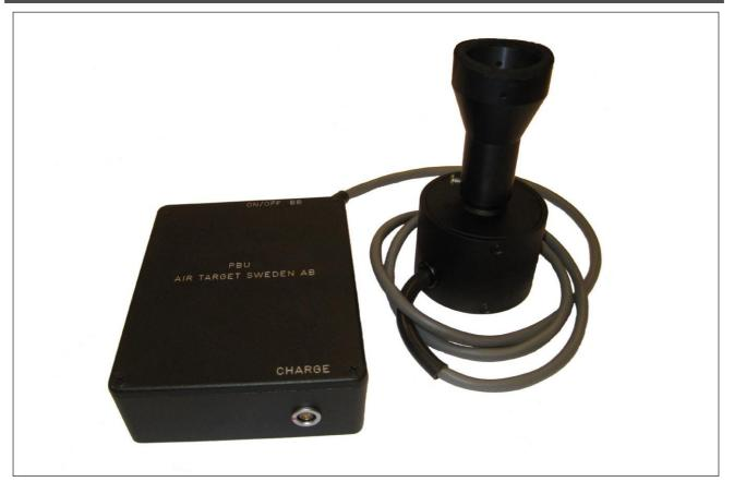
The Portable Bang Unit PBU-2 is a small handy battery operated unit which produces very accurate sound impulses for testing microphone sensitivity, and for adjustment of the electronic circuits of AS-100 Miss Distance Indicators (MDIs).
