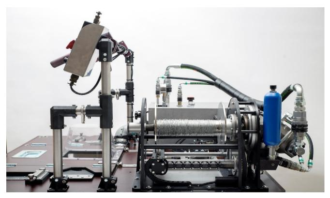
The MBV-45 electro/hydraulic operated winch is intended for medium duty target towing operations with inboard installation in the towing aircraft.
